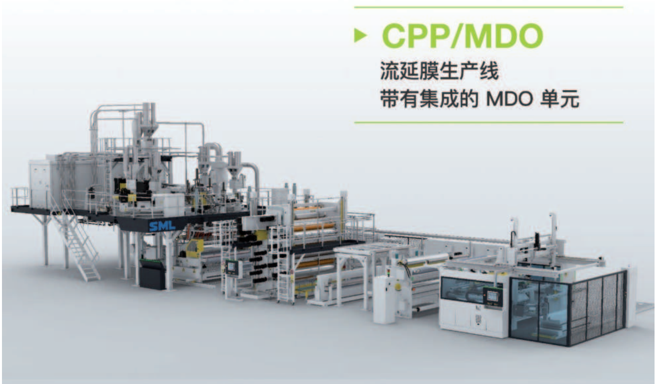
CPP/MDO Cast film line with integrated MDO-unit
